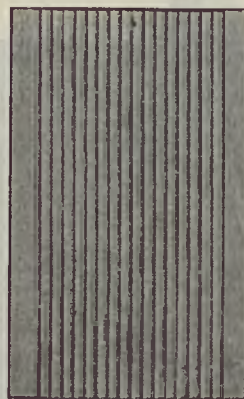
FIG. 21. Grooved Wood Separator — Vehicle and General Service. 1/5 size.
