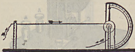
FIG. 7.—Simple Illustrative Model of Hot-wire Amperemeter.
